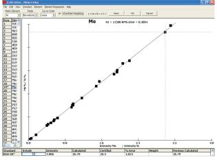
Molybdenum is another major alloying constituent in nickel alloys ranging upwards of 28%. The Mo curve here shows the linear fit with high Mo containing Hastelloy<sup>®</sup> grades of nickel.
