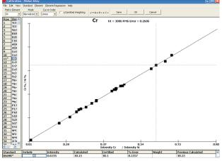
Nickel alloys contain Cr in the range of 0.5% to 30%. The chromium curve demonstrates a linear fit throughout this range.
